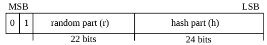
Figure 1: Format of a Resolvable Private Address (RPA). The hash part (h) is generated by a hash function using the random part (r) and a secret key (IRK).
